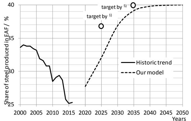
Fig. 2 Share of steel produced in EAF
