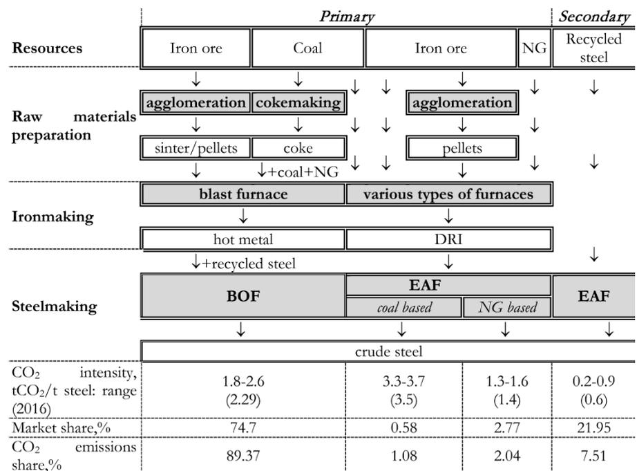
Fig.1 Steel production routes (BOF – basic oxygen furnace, EAF – electric arc furnace, NG - Natural gas, DRI – direct reduced iron)
